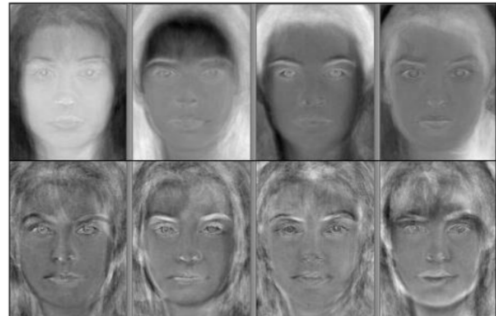
Figure 4: Eigenfaces pertaining to highest eigenvalues (top row) and highest correlations with ratings (bottom row)
